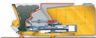
2) Compaction of material (high density)
